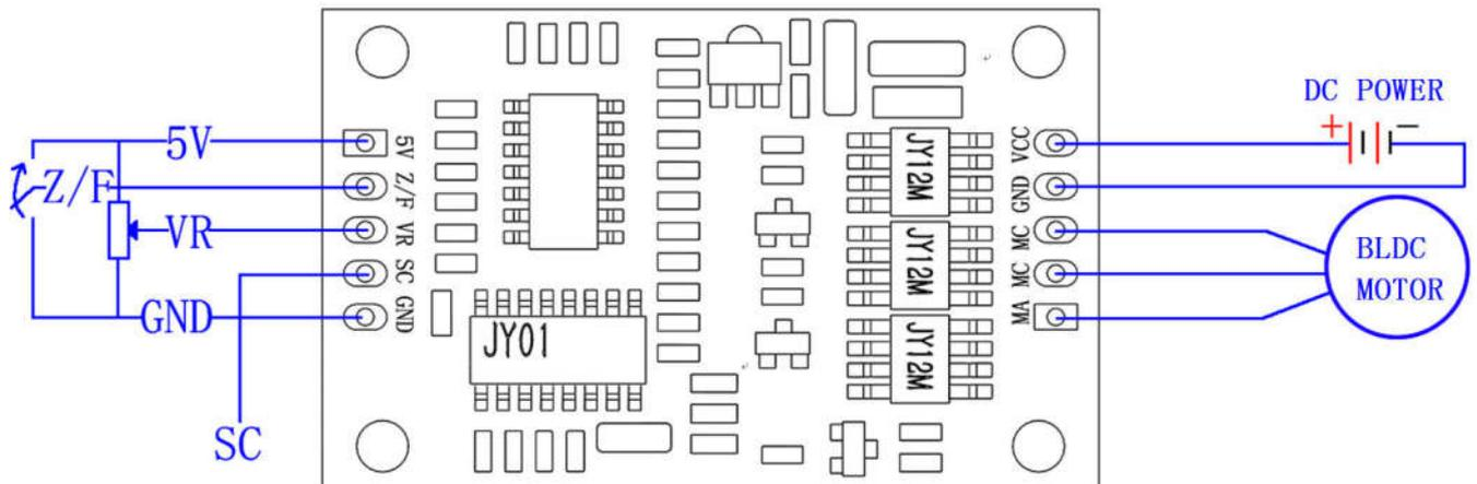
**5V** -----Driver board internal output voltage
